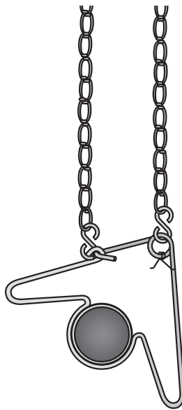
Figure 3.7 • Angled Hanger Mounting Options
