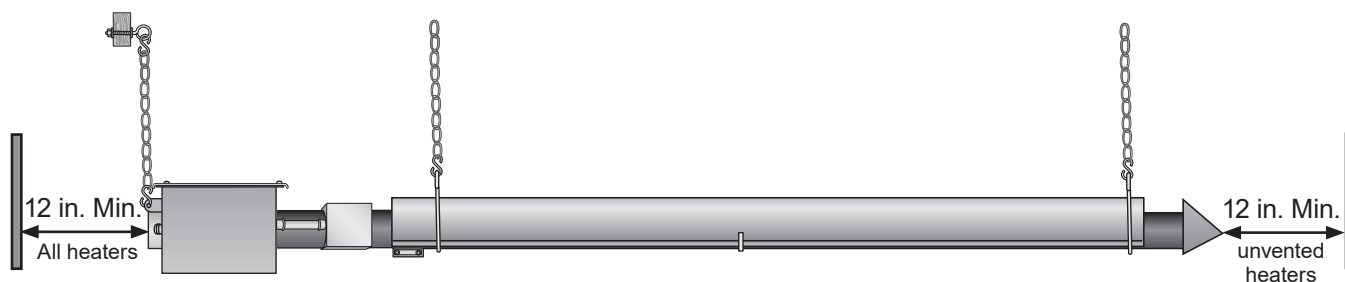
Figure 3.28 • Minimum End Clearances
