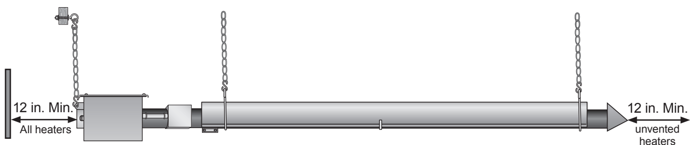
Figure 3.22 • Minimum End Clearances
