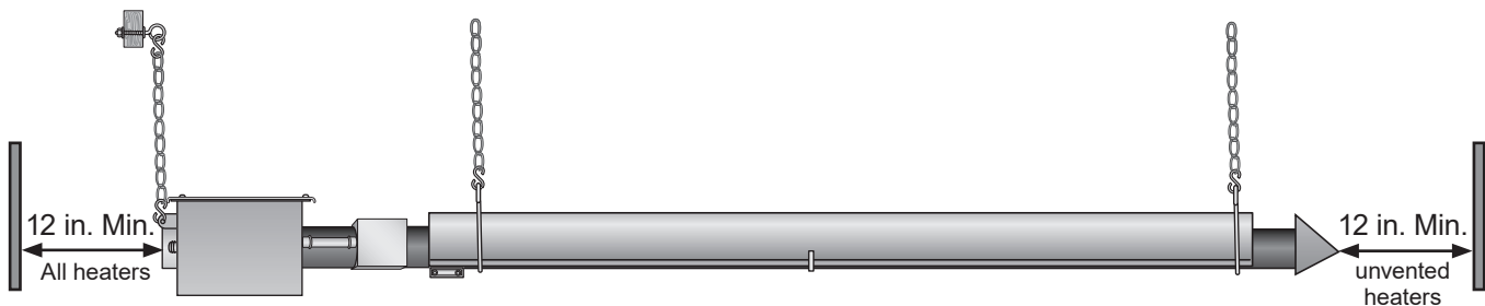
Figure 3.25 • Minimum End Clearances
