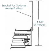
maintained. Clearances are measured from the radiant surface and/or heater bottom to the nearest combustible surface. It is essential that the position and the angle of the installation avoids any possibility of curtains, draperies or other flammable material coming in contact with the heater.
