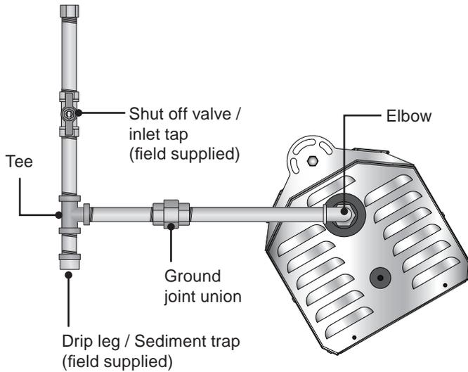
**NOTE:** Do not exceed 14 inches W.C. to the appliance. Use a regulator when gas supply pressure exceeds 14 inches W.C.
