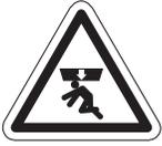
Improper suspension of the infrared heater may result in collapse and persons being crushed. Always suspend from a permanent part of the building structure that can support the total force and weight of the heater.
