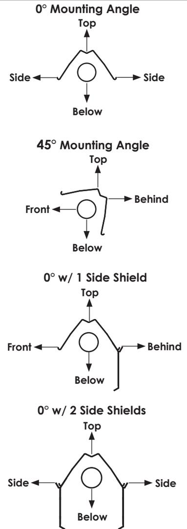
\* Heaters mounted on an angle between 0° and 45° must maintain clearances posted for 0° or 45°; whichever is greater.
