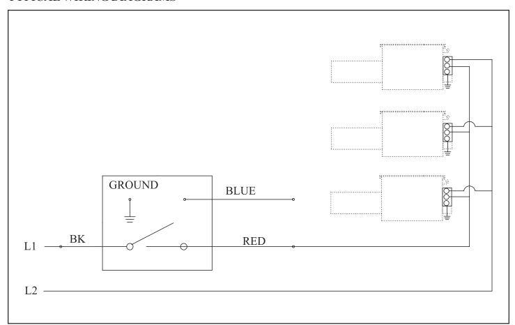
Single or multiple line voltage heaters can be wired to this thermostat. NOTE: Blue wire is used for cooling.
